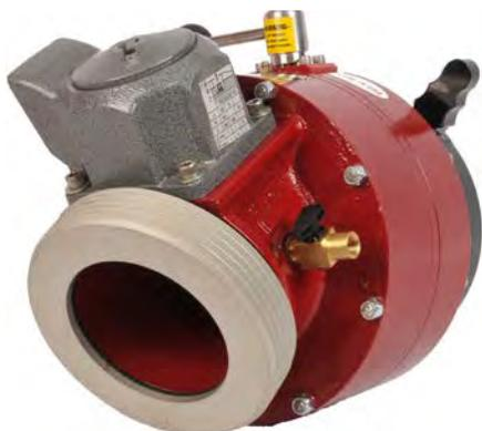
The PRE-CON PC 30 comes standard with a field-adjustable relief valve, large air purge valve at a stress-relieving 30° angle for Storz or large NST hose. The PC 30 only opens as far as necessary for the discharge flow requirements. As discharge lines or nozzles are opened or closed, the PC 30 continually adjusts for changes in water flow. The straight-through design enhances flow and eliminates cumbersome 90° elbows that can interfere with pump controls.
