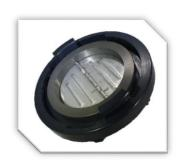
**Description:** Hydra Storz is a quick connecting device that has a built-in check valve feature to protect your hydrant from foreign objects being placed inside. This design allows you to connect up seamlessly to a hydrant without removing caps when used properly. Only time a blind cap would be utilized is when you are pressurizing the hydrant to use the 2.5" steamer port connections.
